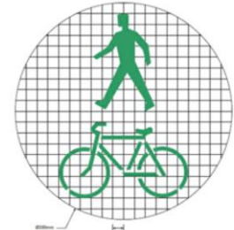
Example: steady green combined walking pedestrian and cycle signal
