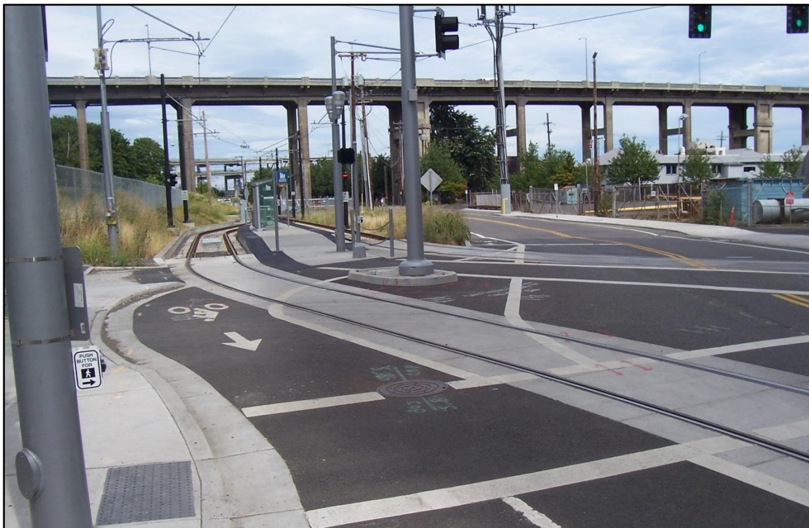
Figure 4-6: A cycle lane is re-aligned to cross a railway closer to 90 degrees (Portland, OR, US)
