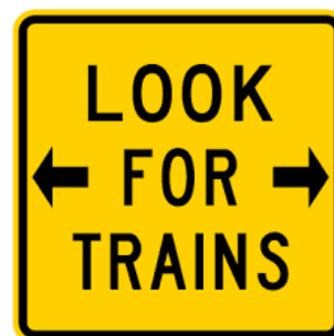
Figure 5-2: Look for trains (WX8) sign
