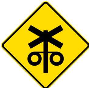
Figure 5-4: Flashing level crossing signals ahead (WX1R) sign
