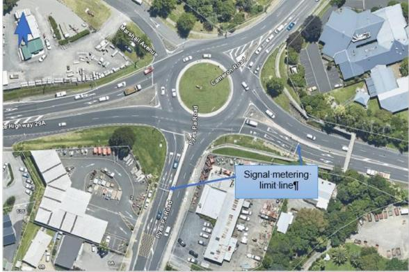
For Barkes Corner, the first design was for three aspect metering signals, for the Pyes Pa Road northbound approach, to provide more through capacity for SH 29A eastbound traffic, to shorten the queue and relieve Takitimu Road Toll Road in the evening peak. Similarly, three aspect metering signals were designed for the SH 29A westbound approach to the roundabout to relieve queues on Pyes Pa Road in the morning peak.
