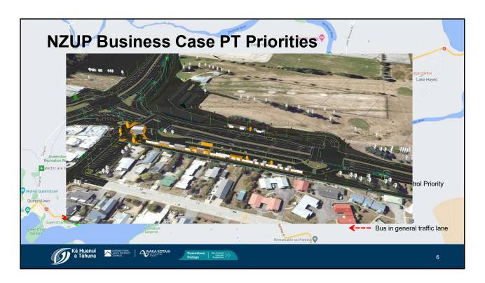
BP is the network pinch point. By signalising we can control the traffic heading into town Marina/Sugar Lane is the only 4 leg intersection on Frankton Road and therefore a constraint on the network; creating new intersection at other end of marina to remove the RT at the existing intersection so now all intersections have roughly equal capacity There MUST be a mode change
