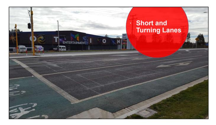
Short lanes are used to separate turning movements from through traffic so they can run separately, to provide additional capacity for turns or to provide a head start for priority traffic such as buses.
