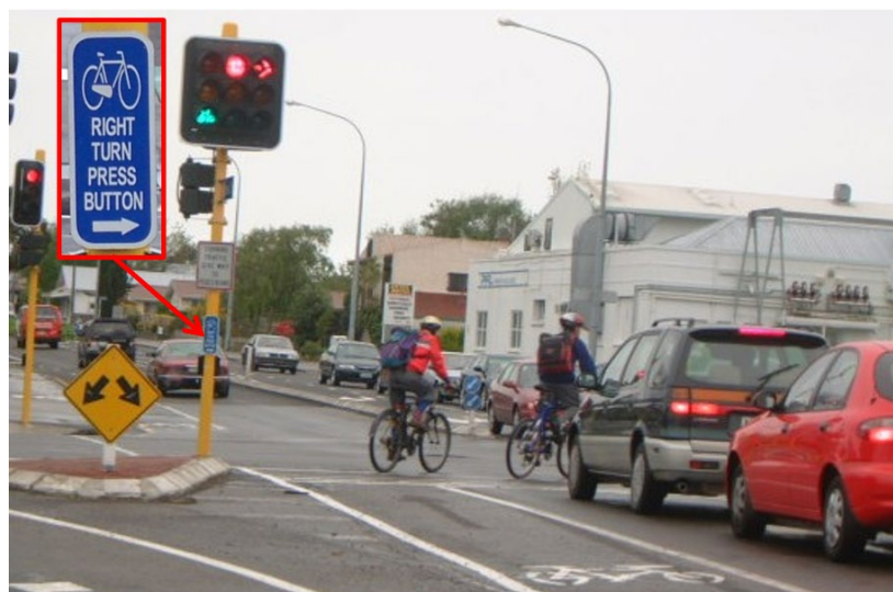
Figure 8-19: Cycle push button used to call exclusive diagonal cycle crossing
