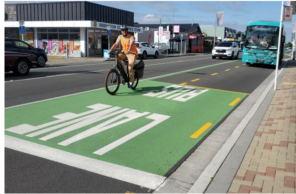
Figure 9-4: Bus lane wide enough for side-by-side use with cyclists, approaching midblock signals
