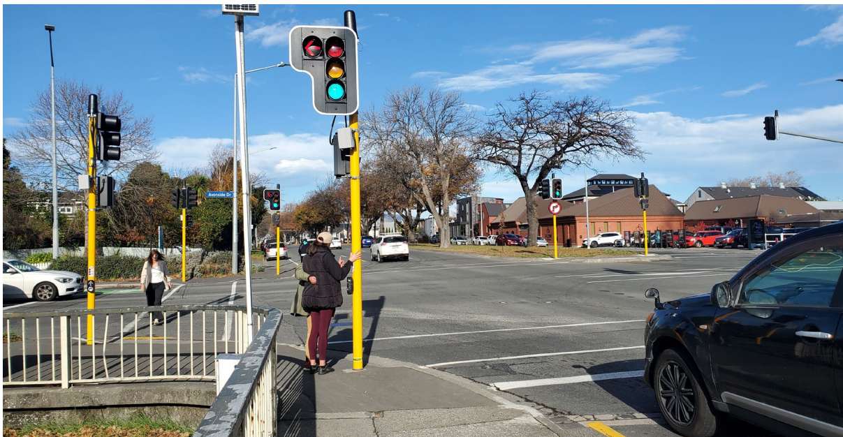
Figure 7-3: Partial pedestrian protection using a red left turn arrow
