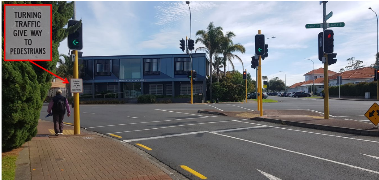
Figure 6-5: Green arrows with no conflict, but “turning traffic give way to pedestrians” sign is misleading
