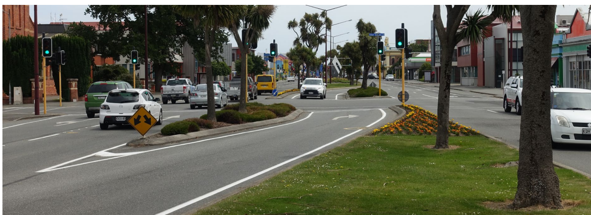
Figure 4-2: Right-turn bays incorporated into solid median achieving excellent forward visibility
